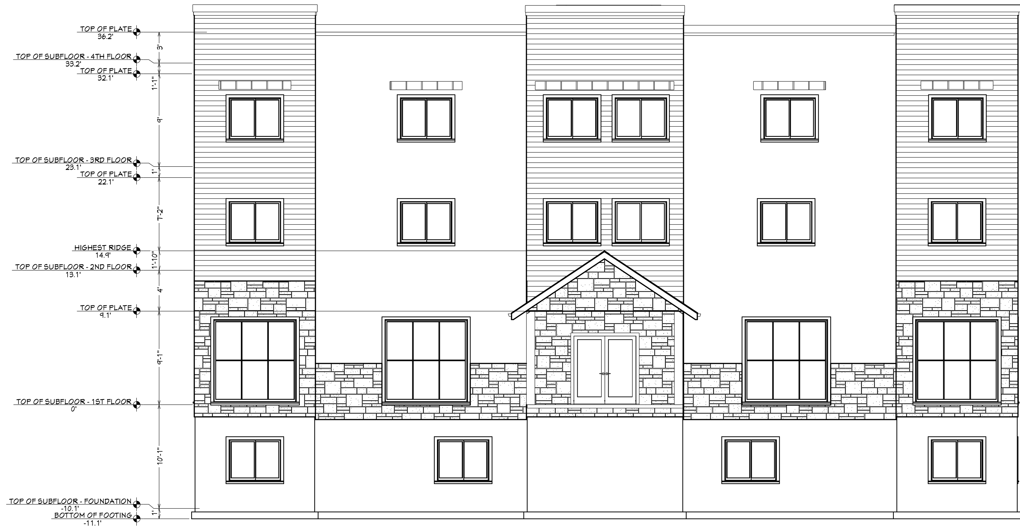
FRONT ELEVATION VIEW 3/16"=1'-0"
