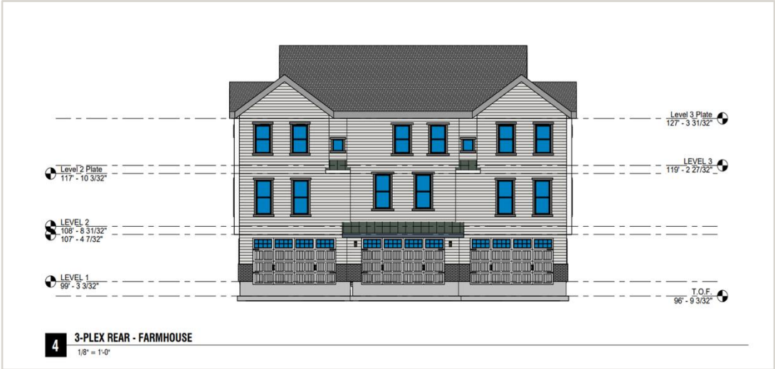
Alley-side elevation — garage doors limit first-story glazing
