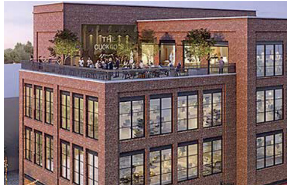
Step Back: a change in the vertical plane of multi-story buildings that preserves the pedestrian experience at sidewalk-level by setting the upper story building facade away from the street
