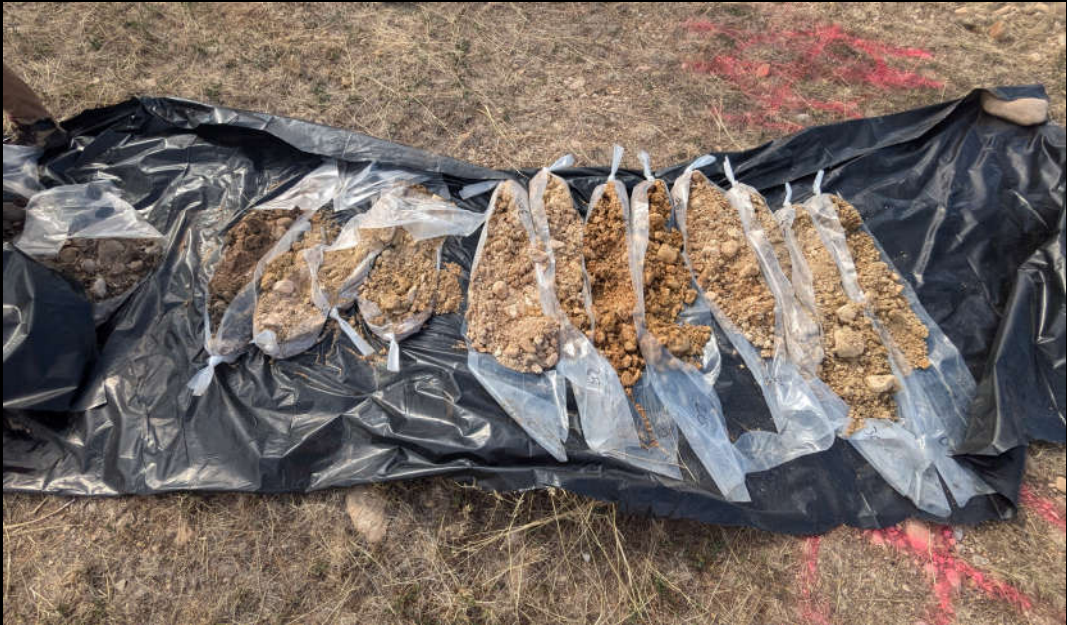
Drilling cores for soil testing. Start of the new runway project
